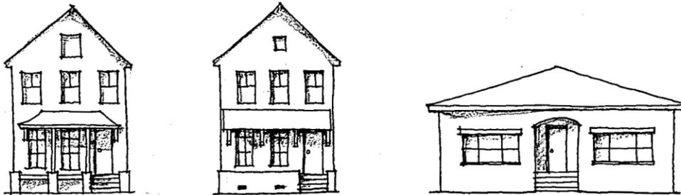
*Directional Emphasis—Inappropriate: Shown above are two houses, typical for the neighborhood and each with a vertical directional emphasis, and a new house that is clearly horizontal in emphasis. This new building is neither sympathetic nor consistent with the established pattern of directional emphasis along this street.*
